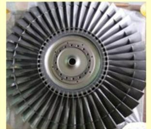
Detonation Spray Coated LPC III modules for Naval Aircraft
